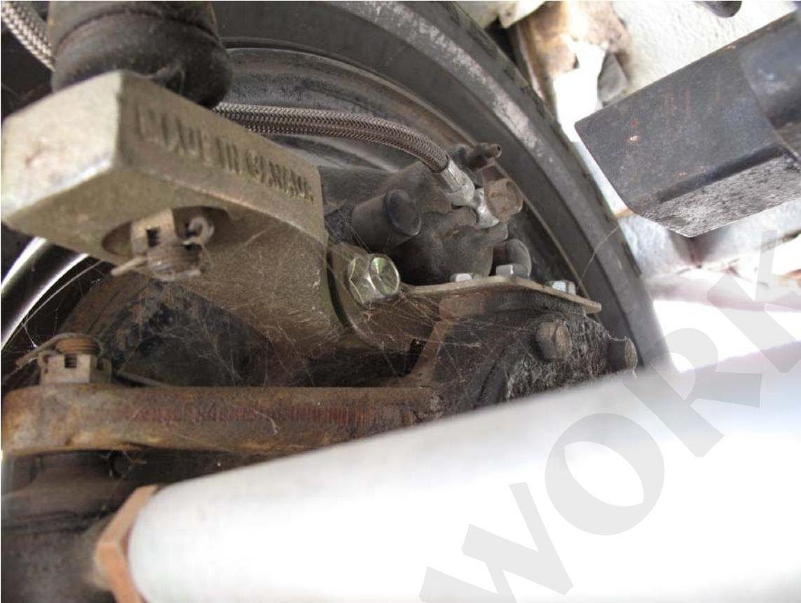
The kit contains a new tie rod and drag link with 2 left thread and 2 right thread rod ends. The rod ends will only fit on 1 end of each rod. Screw the rod ends in and leave them loose.
